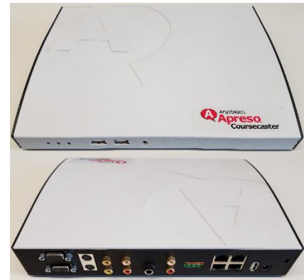
Anystream Apreso Coursecaster – An early generation lecture capture solution may have involved this device, which ingested content and passed it on via the network, but did not actually capture audio or video itself.
