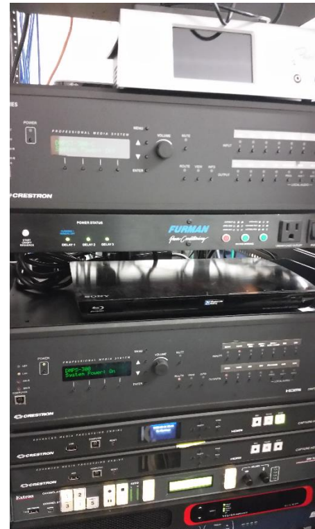
Testing Rack – Our testing rack showing lecture capture appliances from Epiphan, Crestron and Extron.
