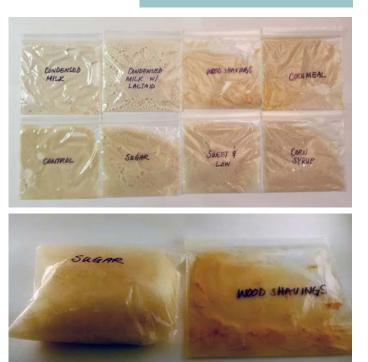
The top image shows the beginning of fermentation after 5 minutes. The bottom image, taken after 20 minutes, shows the bag with the sugar feedstock full of CO2 gas, while the wood shavings bag is flat.
