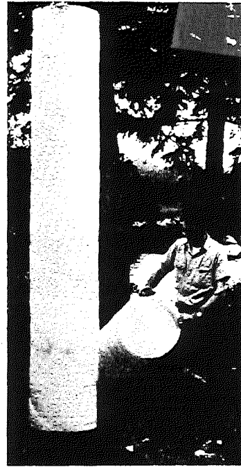
Plankton blooms can be caused by pollution; they lessen the recreational potential of many lakes and reservoirs. The aerators were placed on the bottom of Parvin Lake and were operated 24 hours per day in order to maintain high levels of dissolved oxygen. A stream of air creates currents which draw bottom water to surface.
